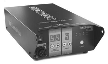
AC/DC Control Unit ref. AC/DC-CPU Compatible with 4LIGHT, 6LIGHT and 4LONG. Can be powered AC or DC.
