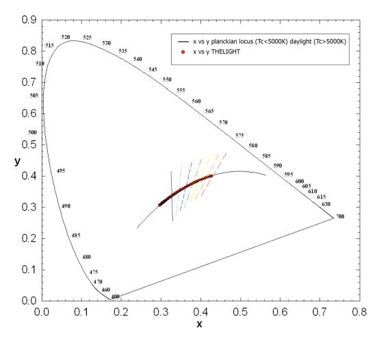
Shown on the diagram are the THELIGHT lamp head chromaticity coordinates (x, y CIE-1931) feed and digitally controlled by its Control Unit and they are compared with the reference illuminants. These reference illuminants are the Planckian locus radiator set below 5000K and the CIE daylight reference is set over 5000K. The Planckian locus radiator references the chromaticity for several tungsten lamps colour temperatures while the daylight locus typify daylight type D illuminants.
